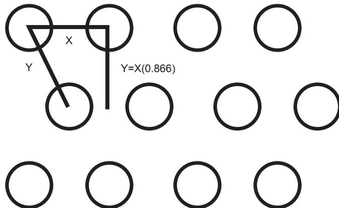
**Fig. 2 - Triangular Spacing**
