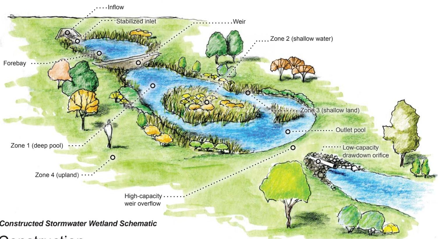
**Constructed Stormwater Wetland Schematic**
