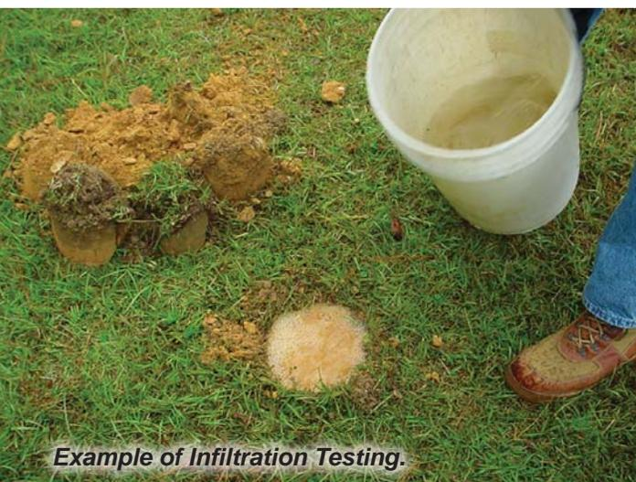
*Example of Infiltration Testing.*
