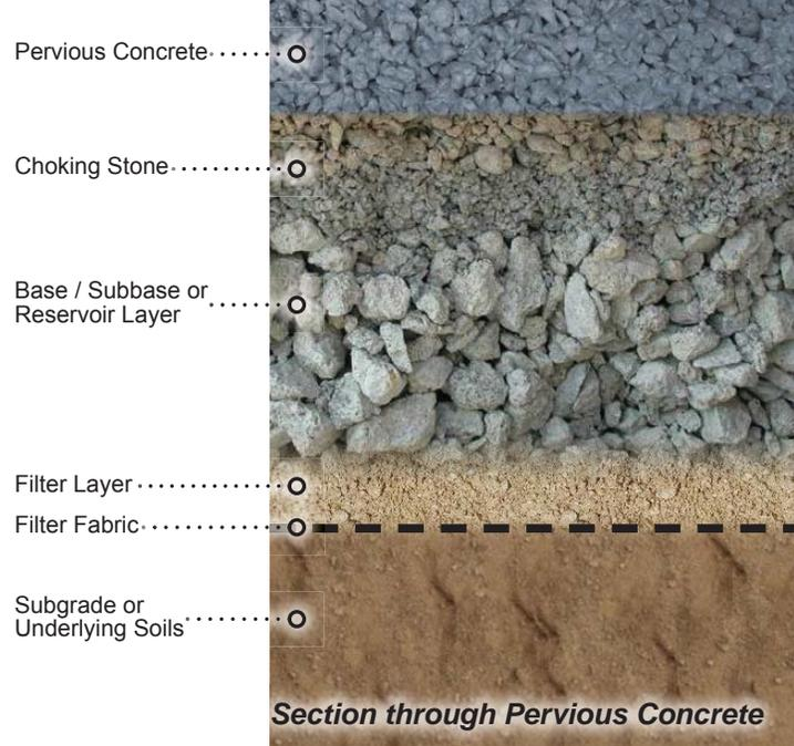
**Section through Pervious Concrete**
