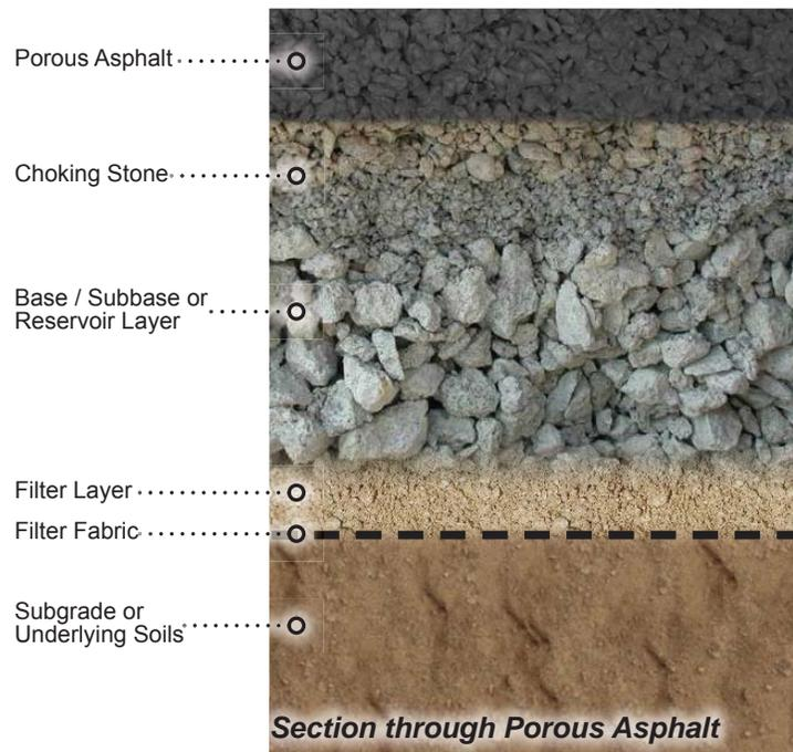
**Section through Porous Asphalt**
