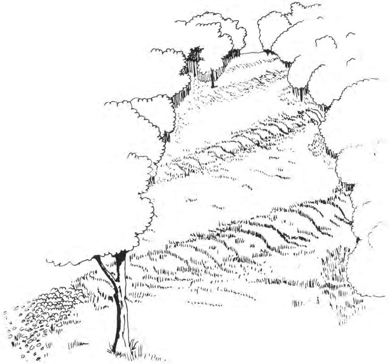
Figure 6.23a Water bars to protect utility right-of-way.
