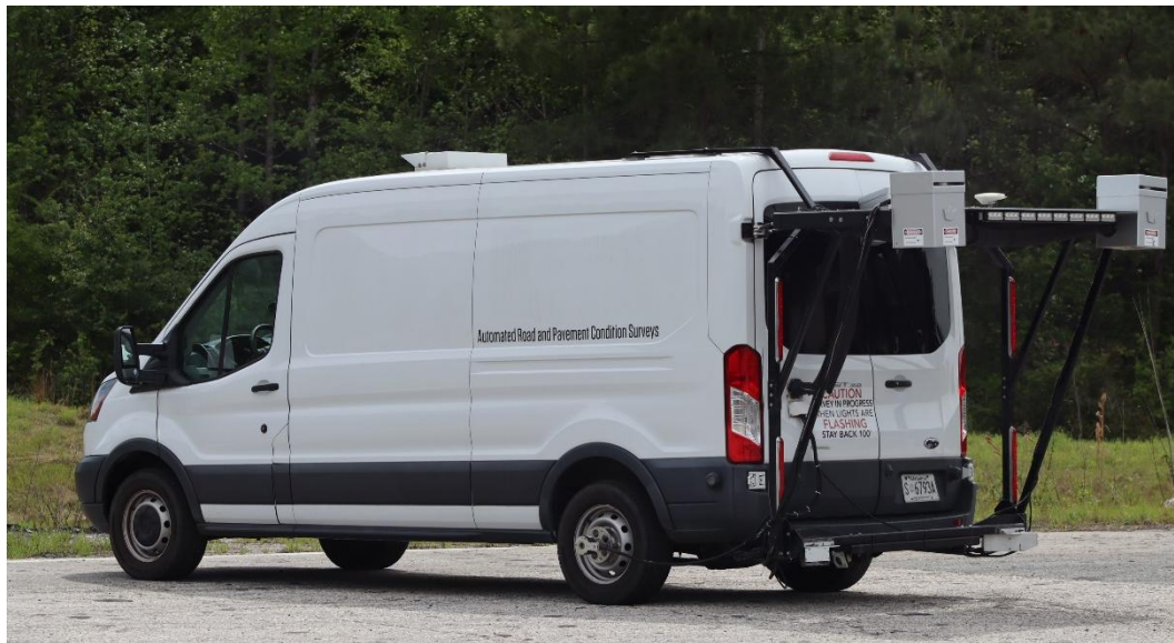
Figure 7. NCAT's Automated Pavement Condition Survey Vehicle
