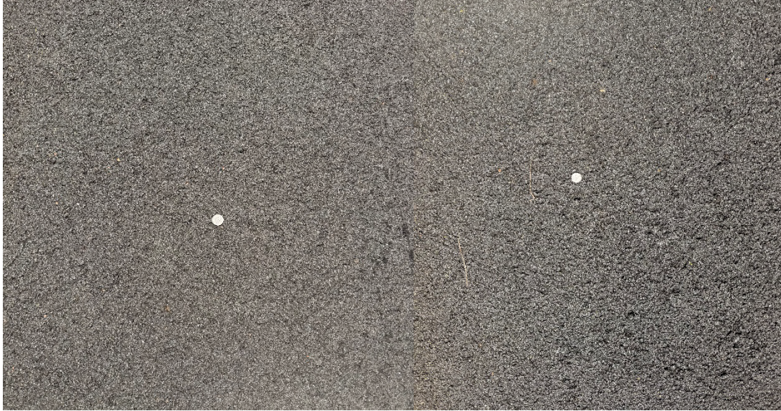
Figure 3 Example of Surface Texture at One-Year (Rubber on left, Control on right)
