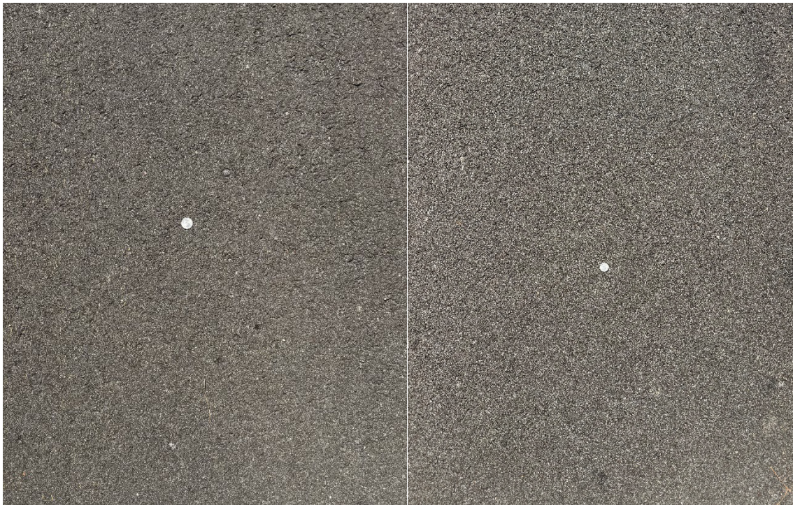
Figure 4 Example of Surface Texture at Two-Years (Rubber on left, Control on right)
