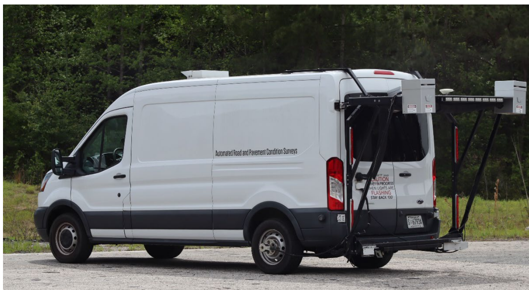
Figure 2 NCAT’s Automated Pavement Condition Survey Vehicle
