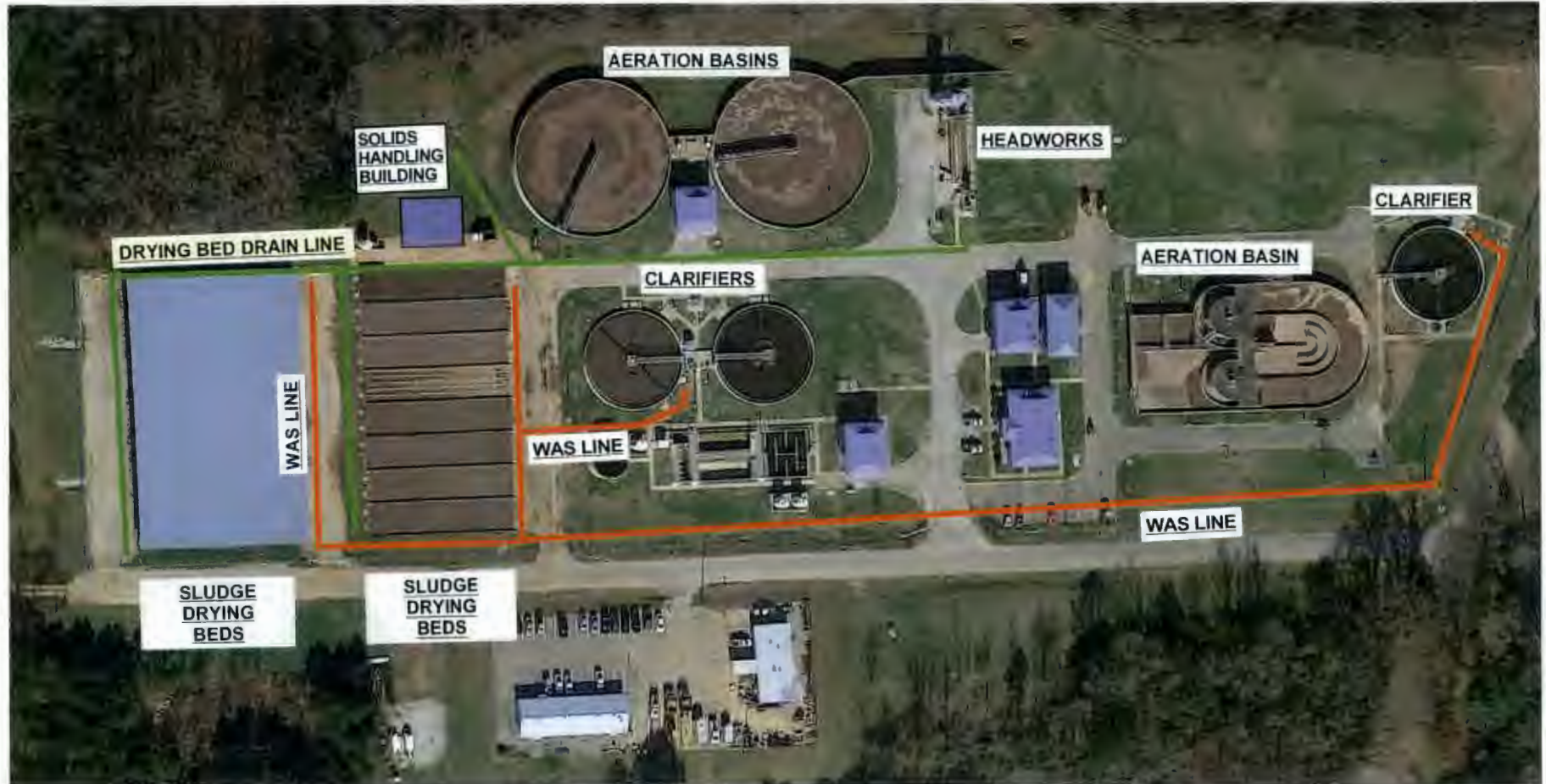
FORM 2S - ITEM 1.15 LINE DRAWING - NORTHPORT WWTP
