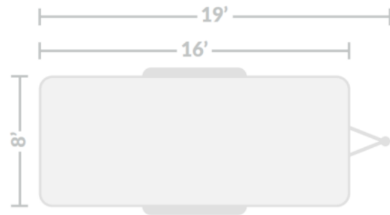
Overhead view of injection trailer dimensions
