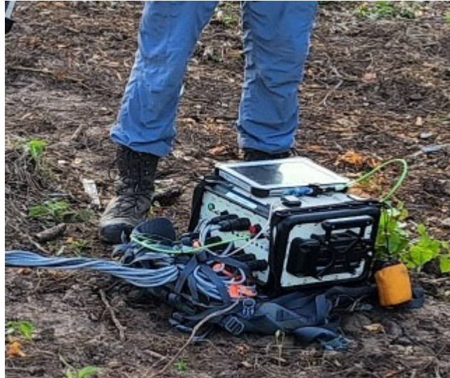
Data acquisition unit with all cables connected
