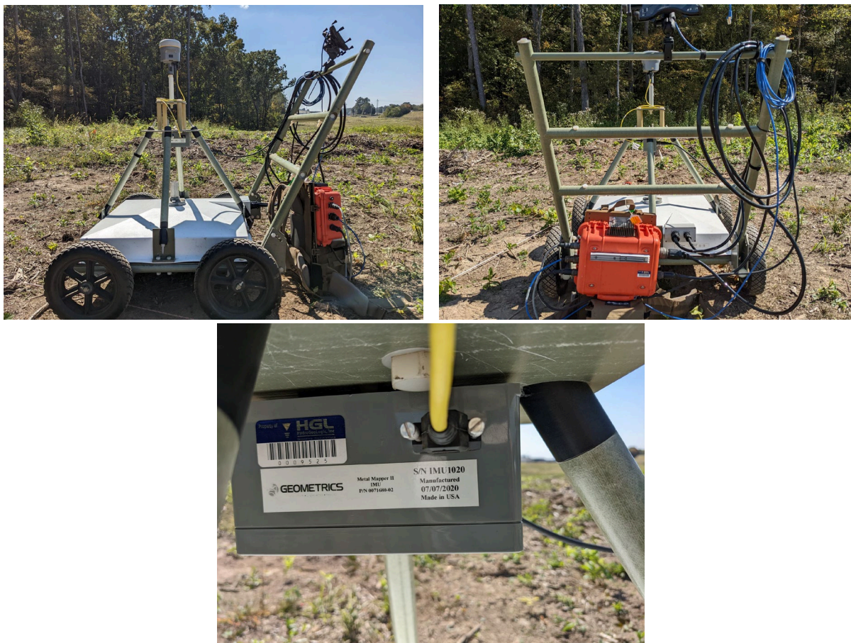
Figure 34. Documentation of MetalMapper2x2 (serial number 1013) assembly at Redstone Arsenal. Full sensor assembly (top left), electronics package (top right), and IMU (bottom).
