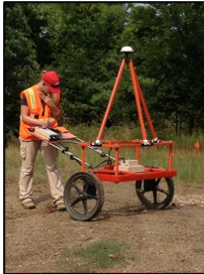
EM61-MK2 wheeled cart configured with WAAS GPS
