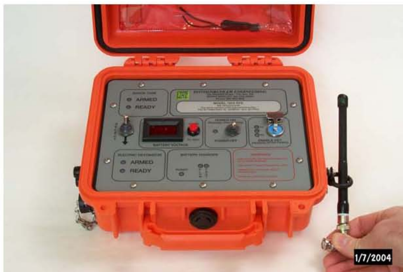
Figure 4-2 Remote Antenna Installation
