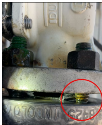
Stud corrosion on flange assembly at Honeywell Geismar after HF release
