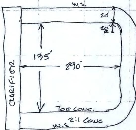
CALCULATING AGITATION REQUIREMENT  $\geq 1841 \text{ #/d}$
