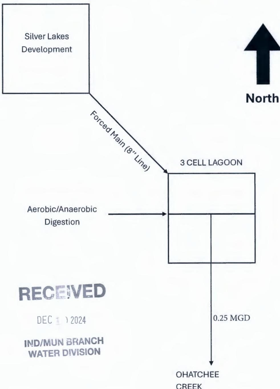
\*Each home has a septic system with a pump that discharges into the forced main line
