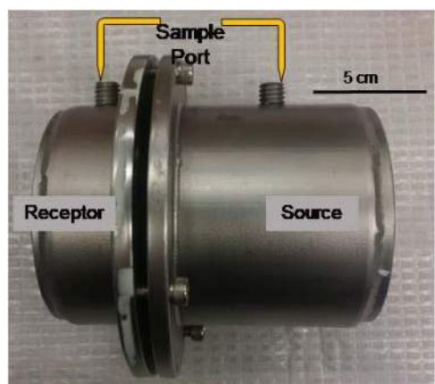
Figure 1: Double Compartment Cell
