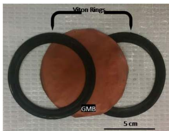
Figure 2: Membrane and Viton Rings
