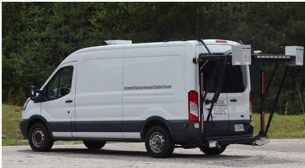
Figure 2 NCAT's Automated Pavement Condition Survey Vehicle
