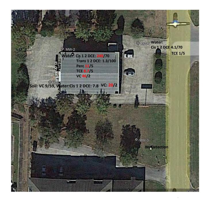
**Legend:** Approximate Boring/MW Location Units: Soil=ug/Kg, Water ug/L
