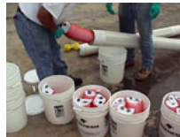
Figure 2. The simple process of loading Filter Socks into Canisters
