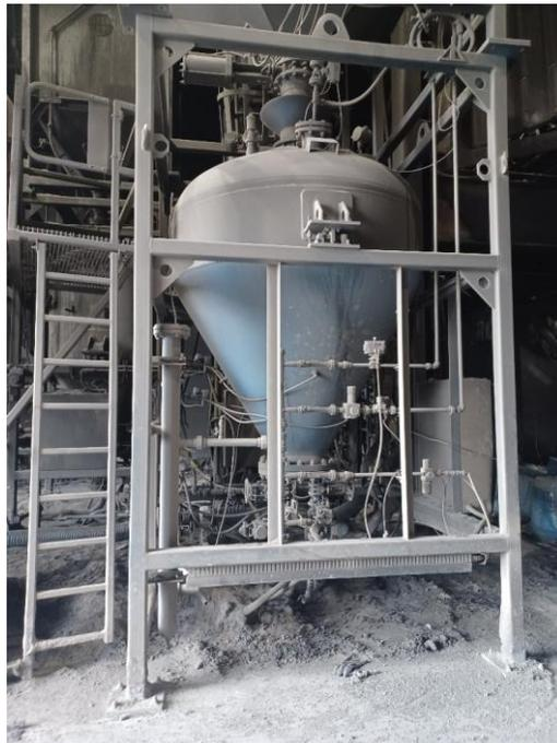
150 cubic ft carbon injector with 200 cubic ft capacity portable hopper
