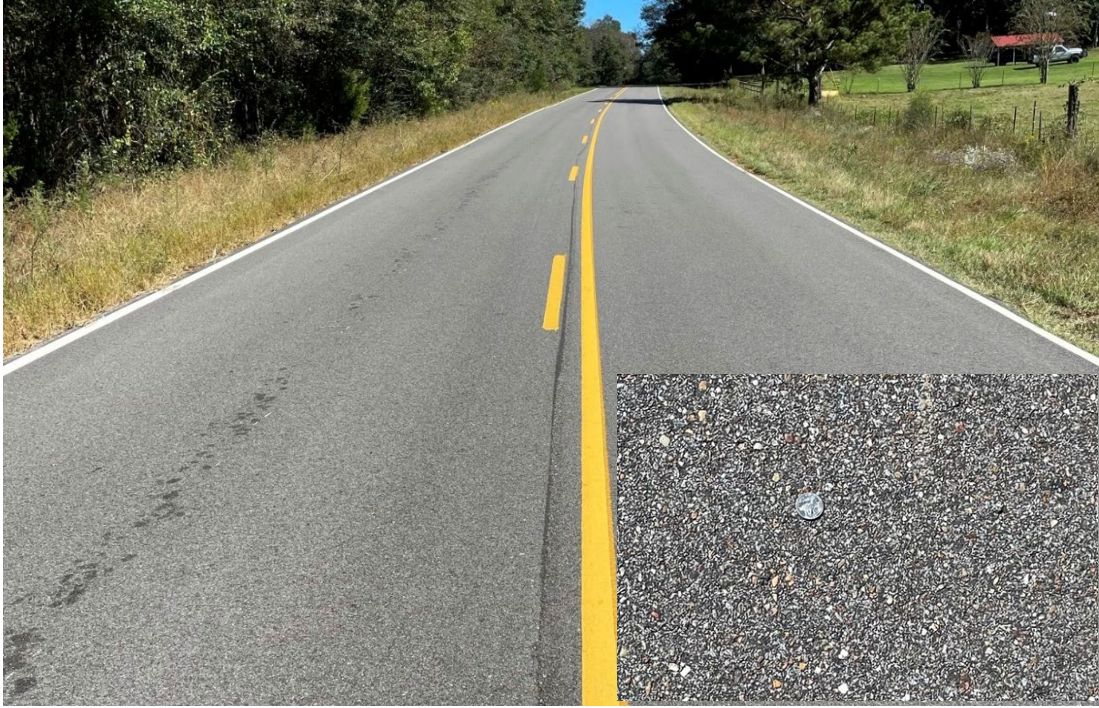
Figure 3 Control BMD Mix at 12-month Inspection.
