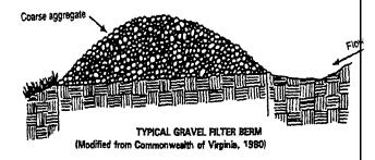
Figure 6 - Gravel Filter Berm
