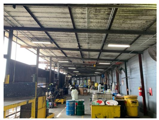
Photo #6: Paint pour off and paint can crushing operation in Building #1.
