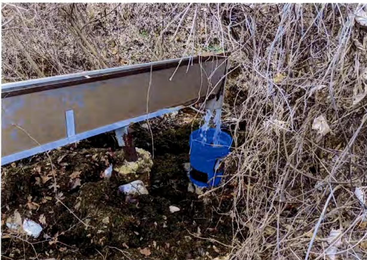
Fish Return Chute and Capture Bucket – 1/17/19
