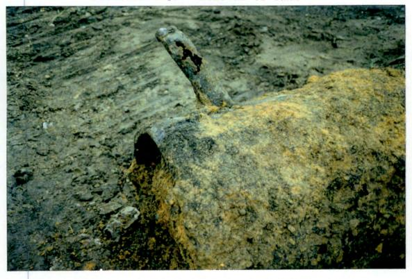
PHOTOGRAPH #6 - Close-up of Hole in Inlet Port Piping
