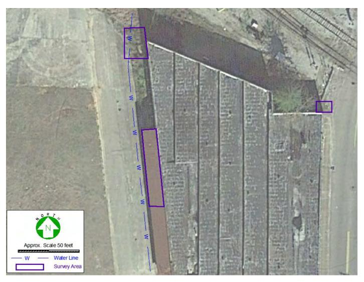
Figure 4: Results Drawing Showing the Location of a Water Line Detected near the Survey Areas.
