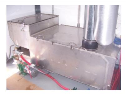
The Stripperator SA20 is a complete process treatment unit for hydrocarbon-contaminated water. It integrates both coalescing oil/water separator and the Cascade low profile Air Stripper into one component. The unit will separate free product, coalesce suspended or colloidal hydrocarbons and settle solids.
