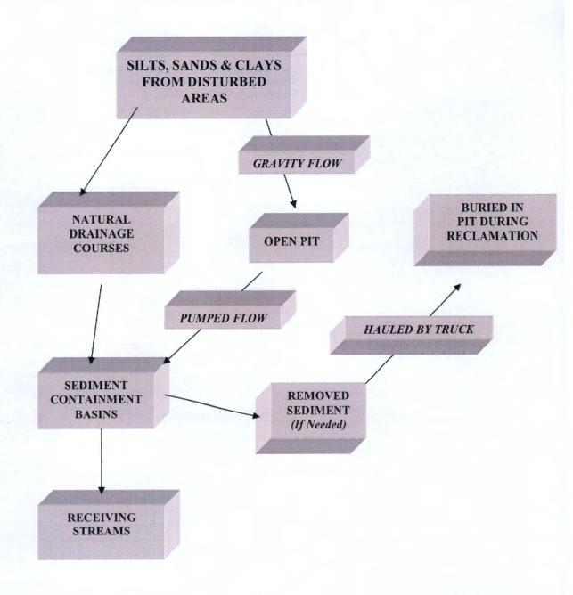
SCHEMATIC DIAGRAM OF WASTE CYCLE
