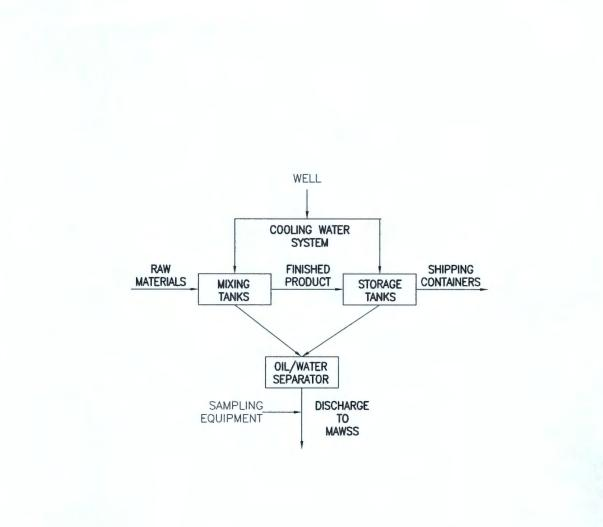
SCHEMATIC OF COOLING WATER MOBILE ROSIN OIL MOBILE, AL
