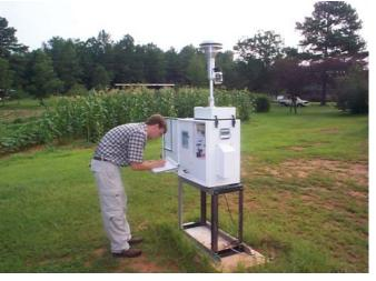
Department perates 60 air moniors at 36 locations throughout Alabama. These air monitors collect ambient air quality data for a variety of pollutants. including particulate matter, nitrogen dioxide, sulfur dioxide, carbon monoxide, lead and ozone.
