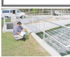
Department inspectors collect samples of the treated water being discharged with a wide variety of manual and automated sampling devices. The water samples can be analyzed for field parameters on site or transported to one of ADEM's three laboratories for analysis.
