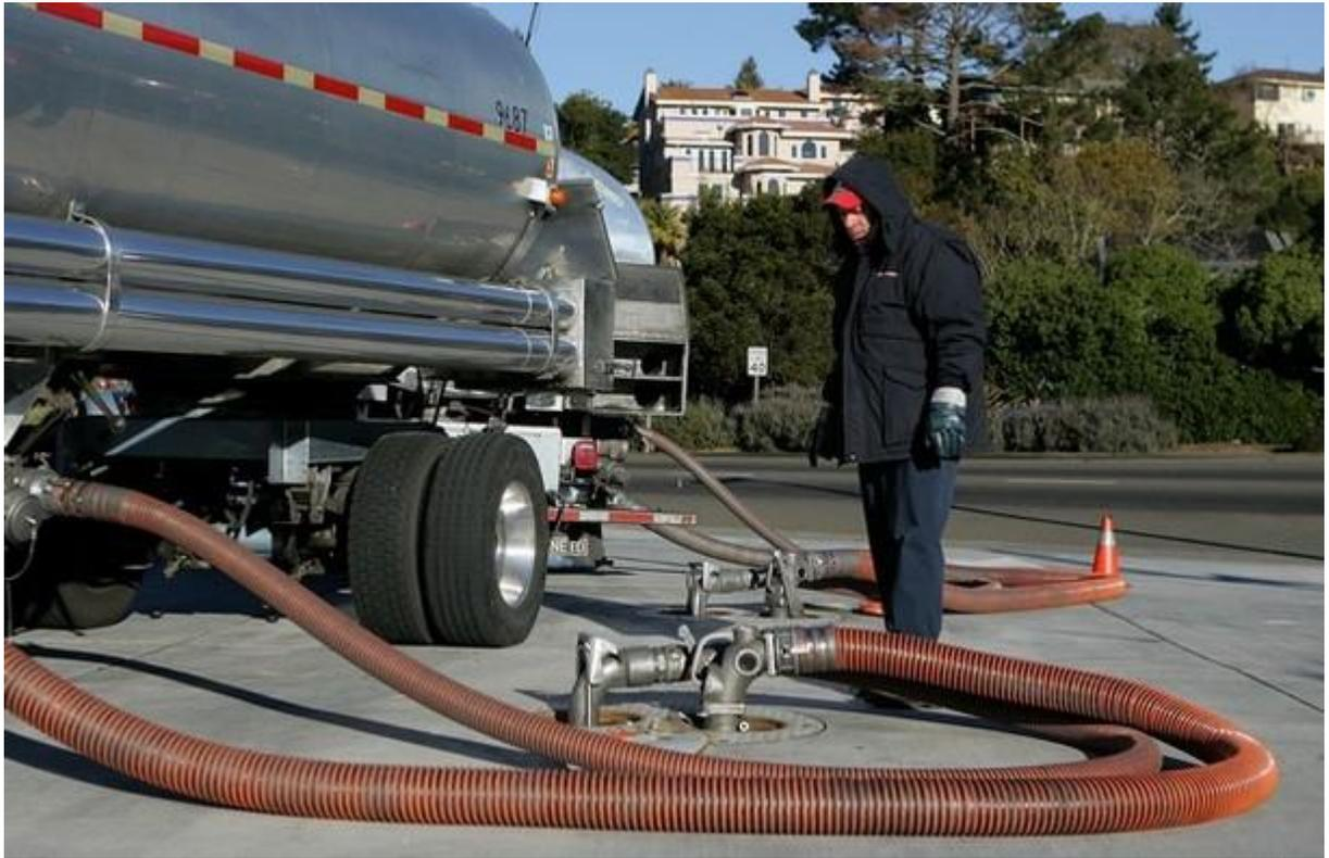
When a truck is dropping gas, remember to always make sure that two (2) hoses are used. One hose should be attached to the fill port, and the other should be attached to the vapor port. If you see ANY fumes or smell excessive gas odors, then inspect the adaptors for proper “hook up” and check the hose wall for tears and cracks. Also, please remember to look up at the pressure relief valves if possible to check for visible vapors.
