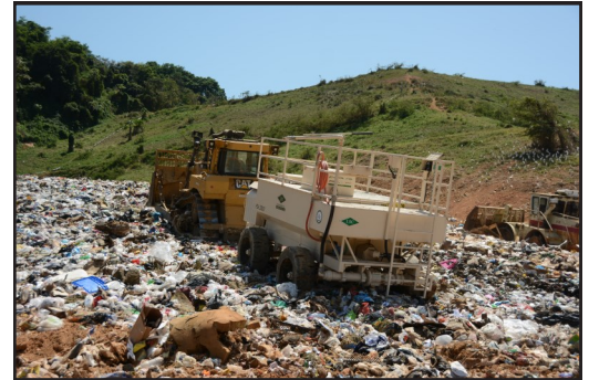
Proper orientation of equipment on slope
