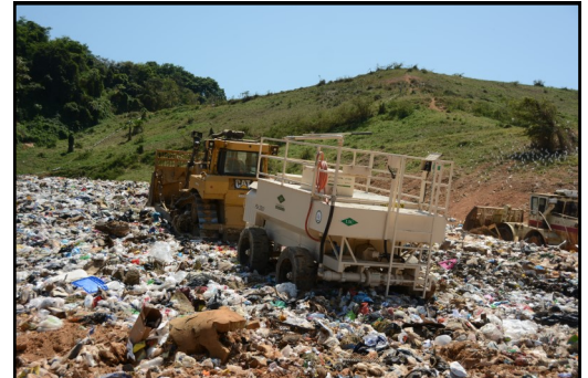
Proper orientation of equipment on slope
