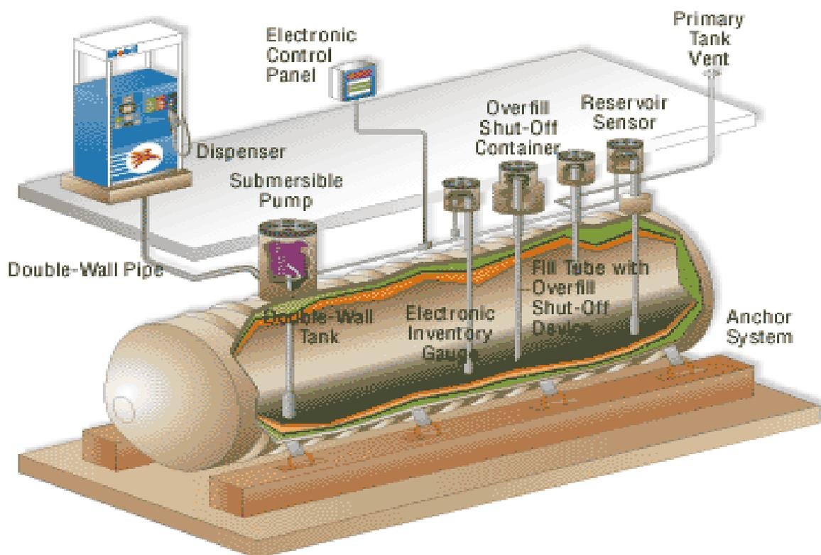
*\* It should be noted that this is an example of an UST system configuration. The system layout may vary from site to site.*
