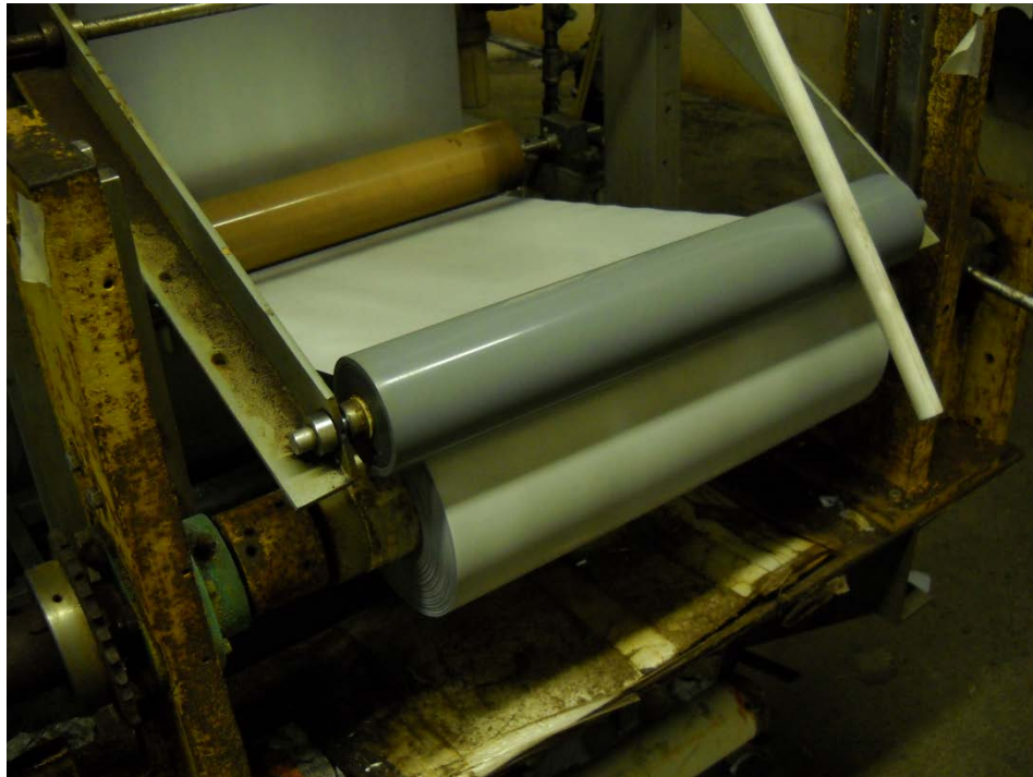
Aluminum foil rolls in etching machine
