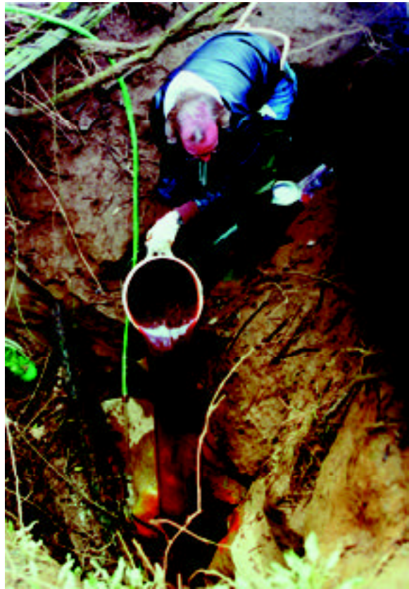
Wellhead protection study. Pouring nontoxic dye for an aquifer time-of-travel test (dye tracing).
