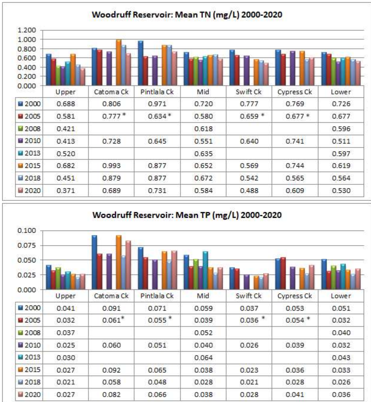
Figure 2. Growing season mean TN and TP concentrations measured in Woodruff Reservoir, April-October, 2000-2020. Bar graphs consist of mainstem and embayment stations, illustrated from upstream to downstream as the graph is read from left to right.
