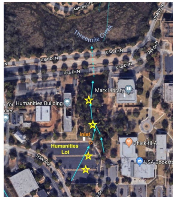
Figure 39. Stormwater path across the humanities parking lot into Three Mile Creek
