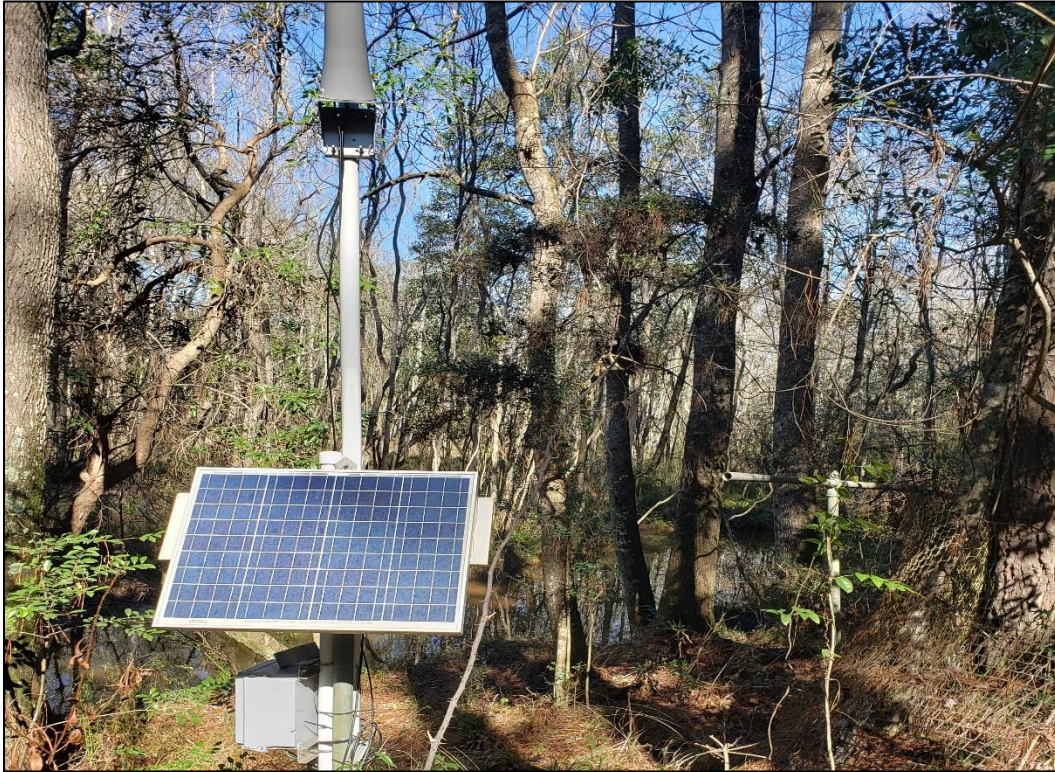
Figure C.5 Joes Branch Station JOBB-2: Continuous In-Situ Turbidity Station
