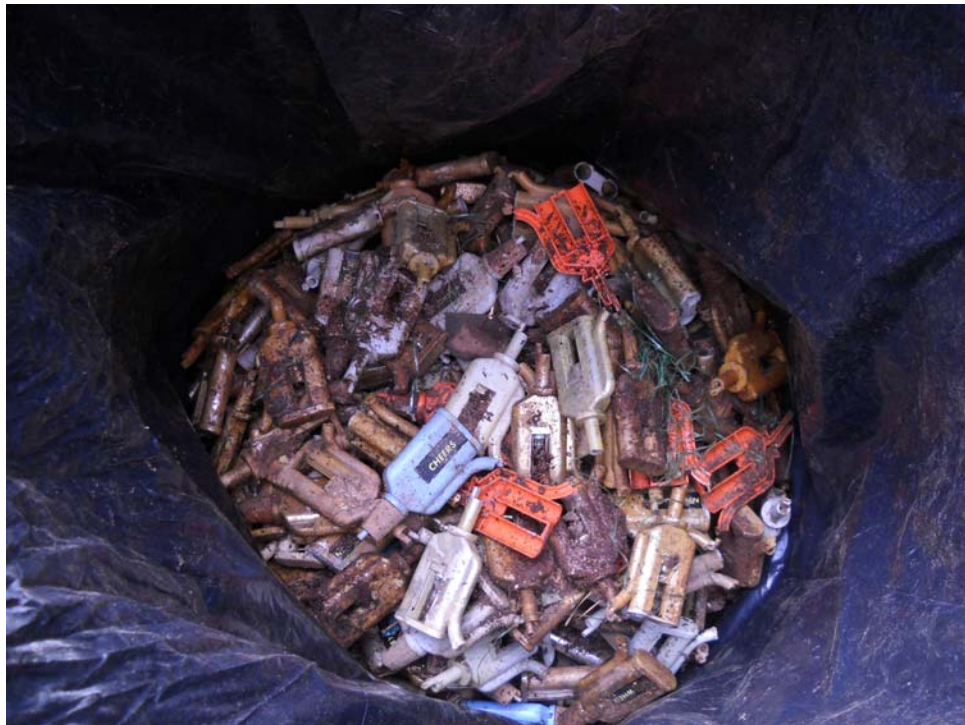
Mercury switches collected and awaiting disposal
