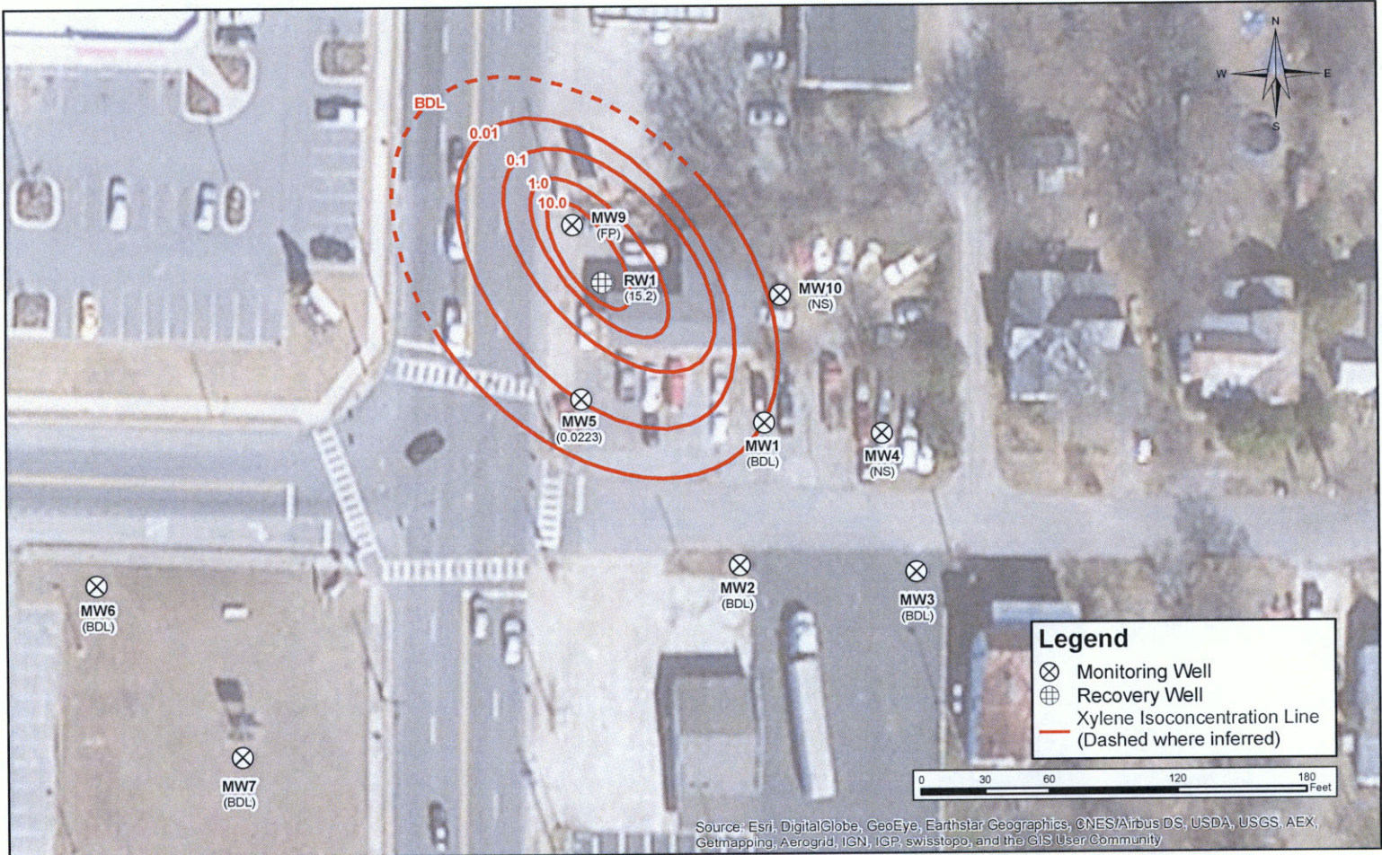
Figure 6 - Xylene Isoconcentration Map Calera, Alabama Calera Garage CP41 Project Number: 1077-009-41 Project Manager: Bob White Date: 3-22-2016
