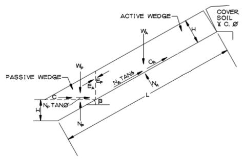
Figure 1, Slope Geometry & Free Body Diagram
