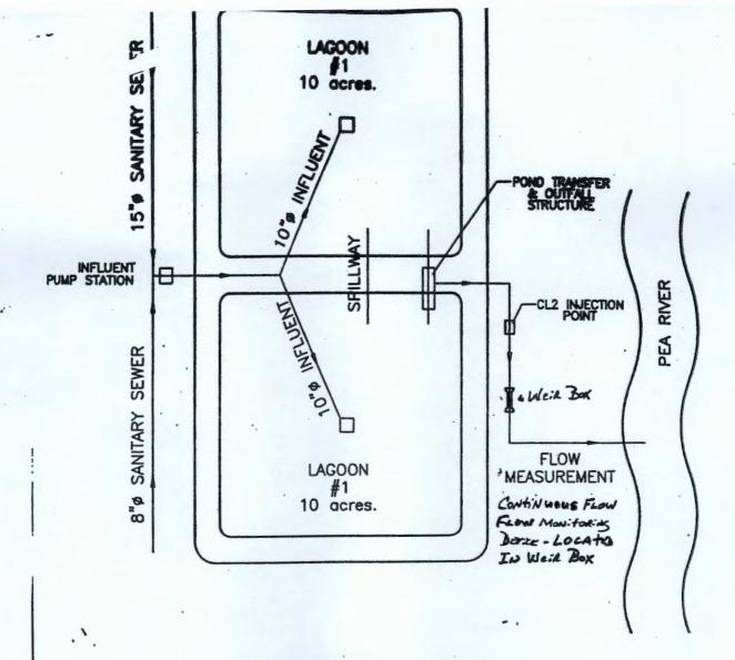
TOP OF EMBANKMENT: 197.24 HIGH WATER LEVEL: 190.24 NORMAL WATER LEVEL: 188.24 BOTTOM ELEVATION: 185.24
