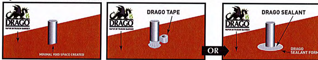
Fig. 4a: PIPE PENETRATION SEALING
