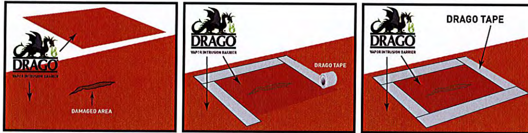
Fig. 3: SEALING DAMAGED AREAS
