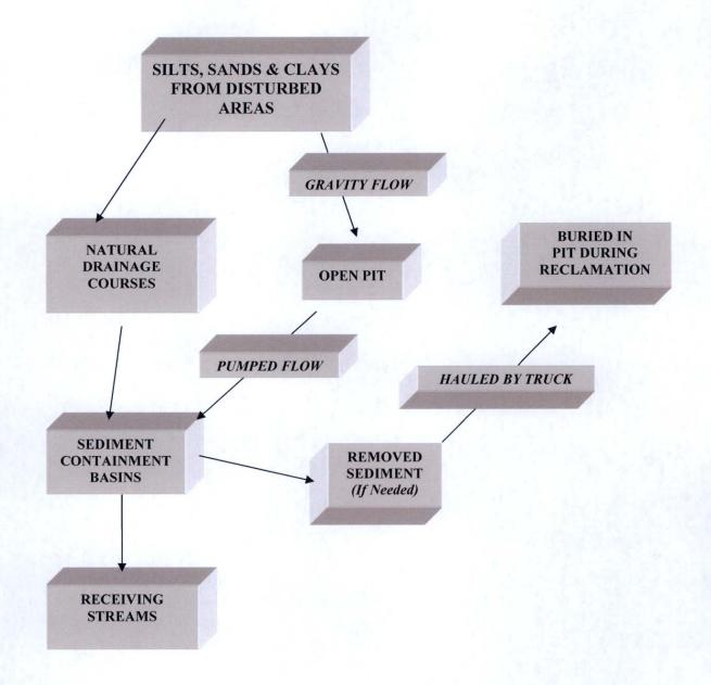
SCHEMATIC DIAGRAM OF WASTE CYCLE
