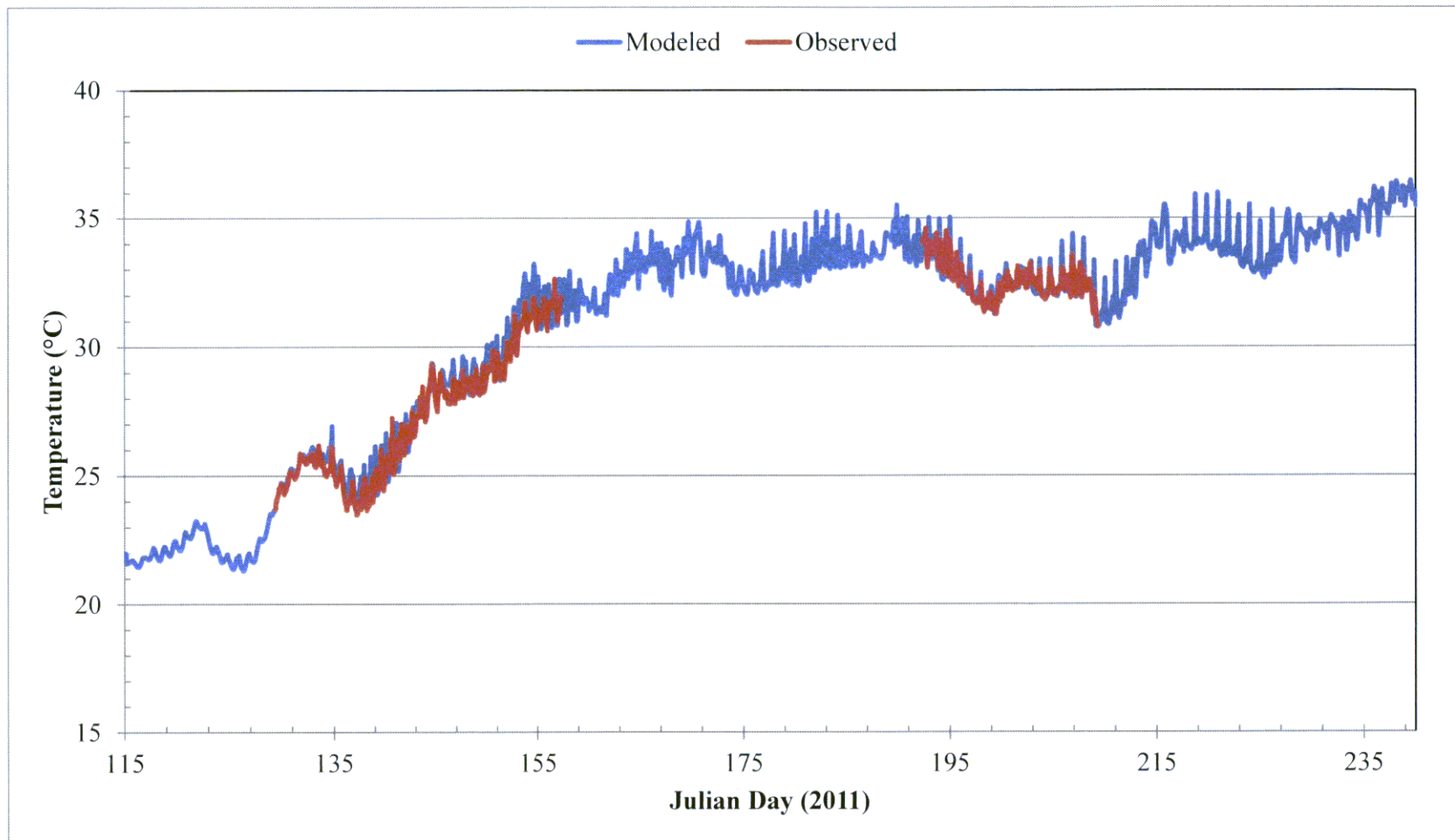
Figure 3.25 Time-series plot of observed and modeled water temperature ( ^{\circ}\text{C} ) at the shallow depth of the macroinvertebrate plate Station 17 from April 26 to August 29 (Julian day 115 to 240), 2011.
