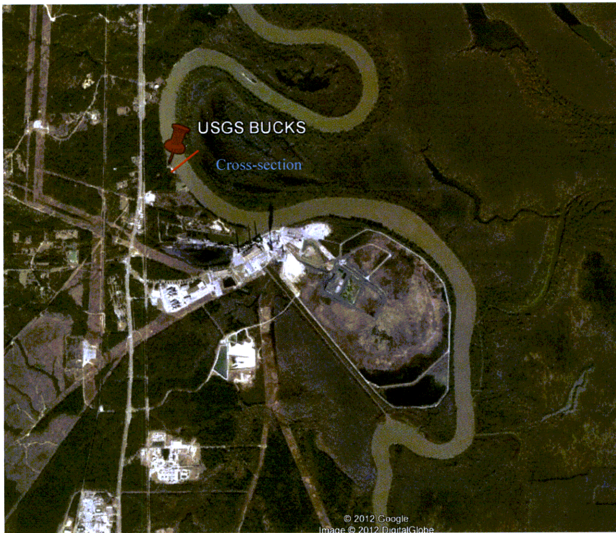
Figure 2.3 Upstream boundary location of the Barry EFDC model – USGS Bucks gaging station on the Mobile River.
