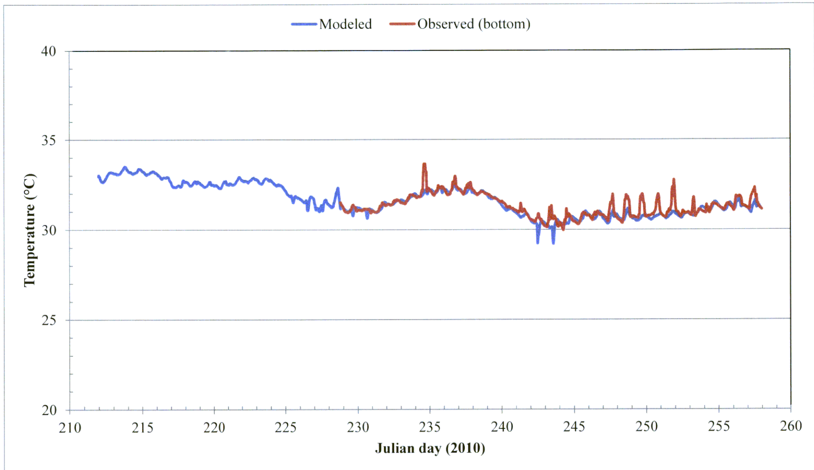
Figure D.4 Time-series plot of observed and simulated bottom-layer ( deep ) temperatures from August 1 to September 16 (Julian day 115 to 284) in 2010 in the intake canal for units 1–3 .
