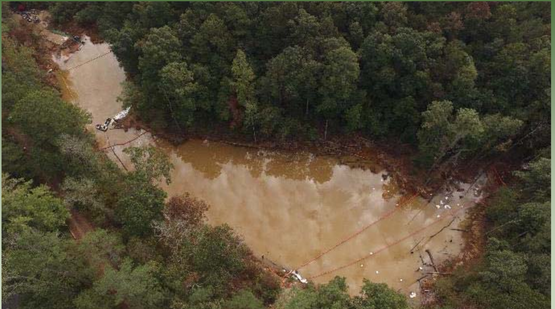
Aerial showing reduction in fuel coverage and installation of protective shore boom.
